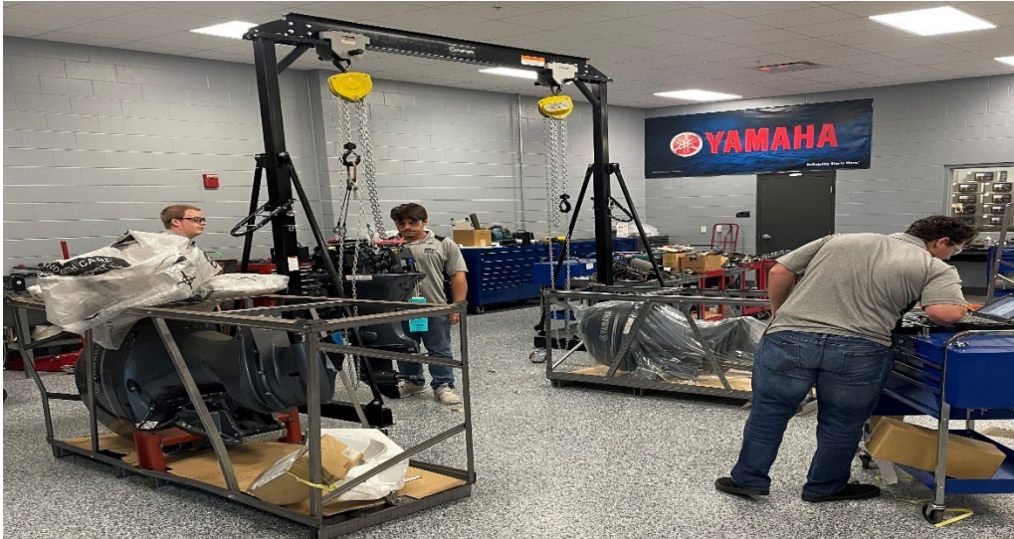
Students in OCP-C uncrating a Yamaha outboard and mount it on an engine stand.
