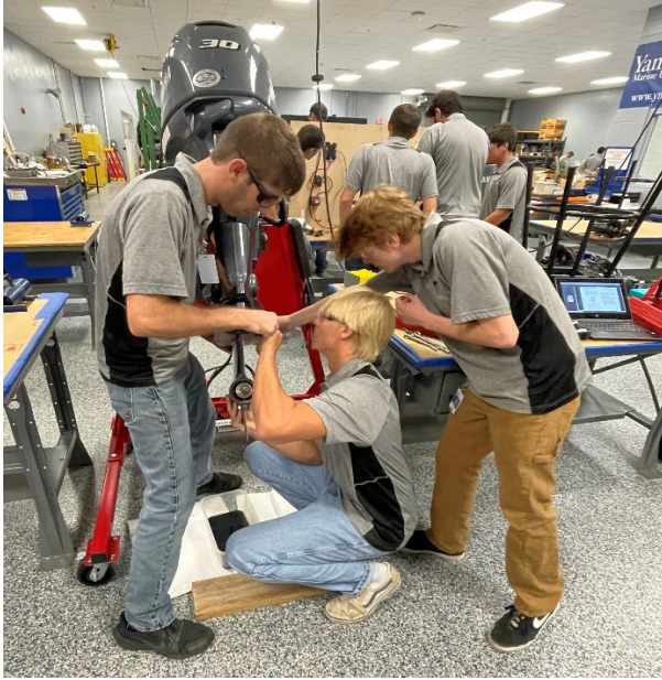
During Critical Thinking Skills students conduct maintenance on a lower gearcase.
